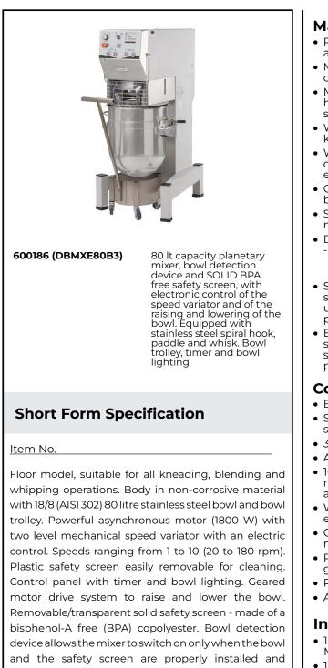
positioned together. Equipped with motorized bowl and bowl trolley. Supplied with 3 tools: stainless steel spiral kneading hook, cast aluminium paddle and stainless steel wire whisk.
